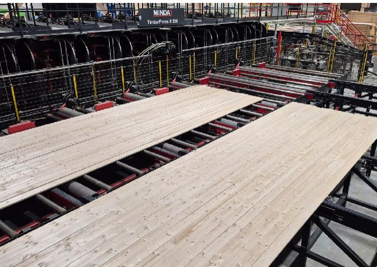
With regard to the press, Arcwood opted for a TimberPress X 336. This press allows the production of elements up to 15.1 m length, 3.6 m width and 340 mm thickness.
