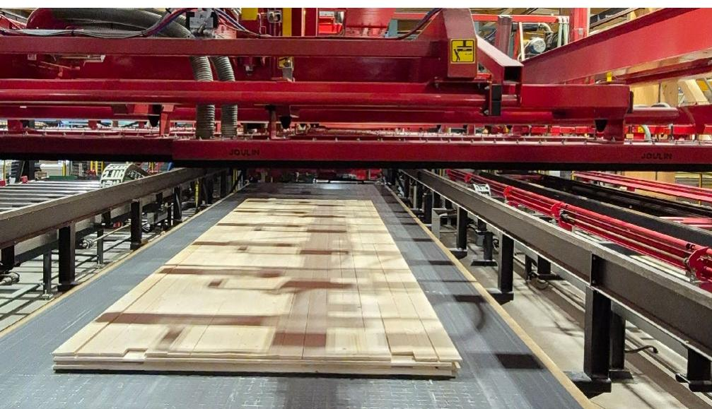
A vacuum portal takes the task to build the layer. This is followed by gluing.
