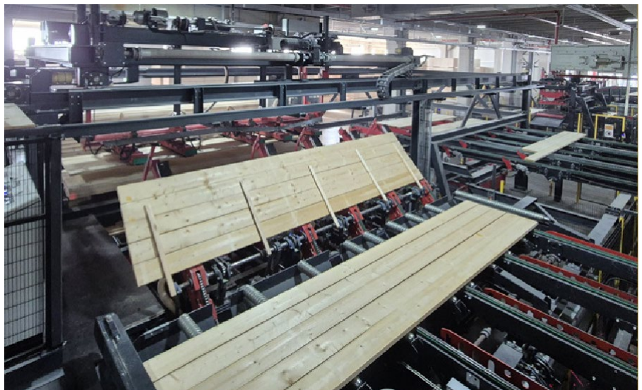
The bars are tilted during vacuum destacking
