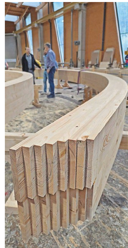
Large, complex glulam beams for such large timber-construction projects are the specialty of Huter & Söhne
