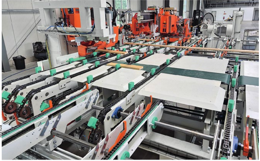
The DuoZink12 finger-jointing machine during pre-commissioning at MINDA
