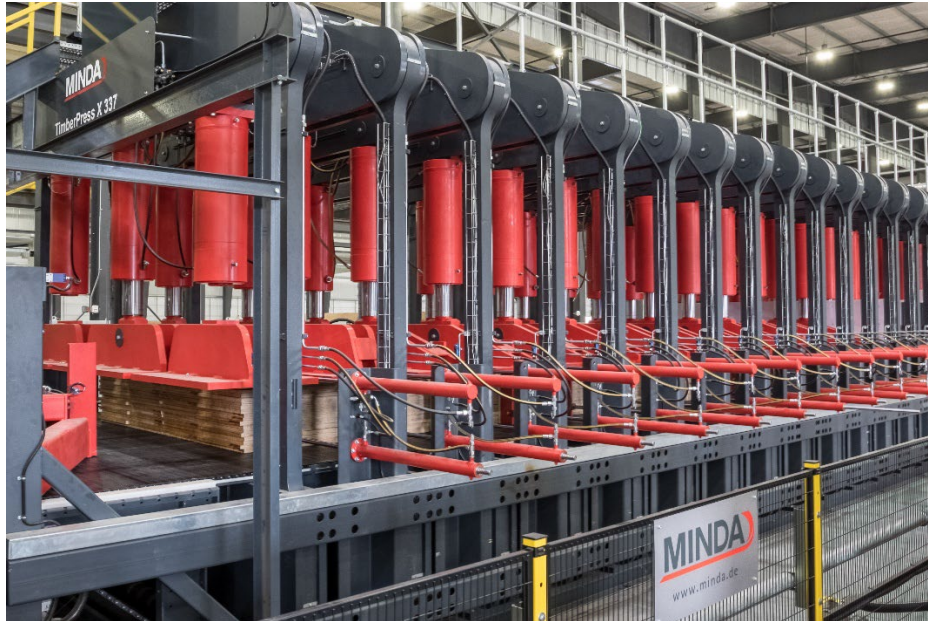
MINDA has modified the TimberPress V 120 glulam press to produce split beams
