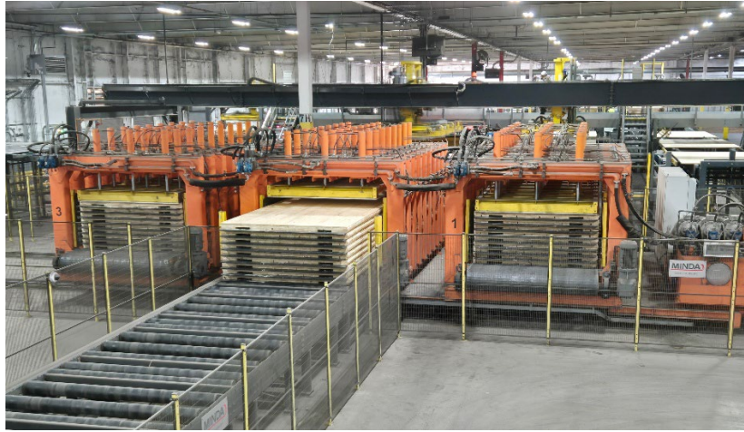
Three CLT presses type TimberPress X 224 in operation at Sterling. The finished panels leave the lines every minute
