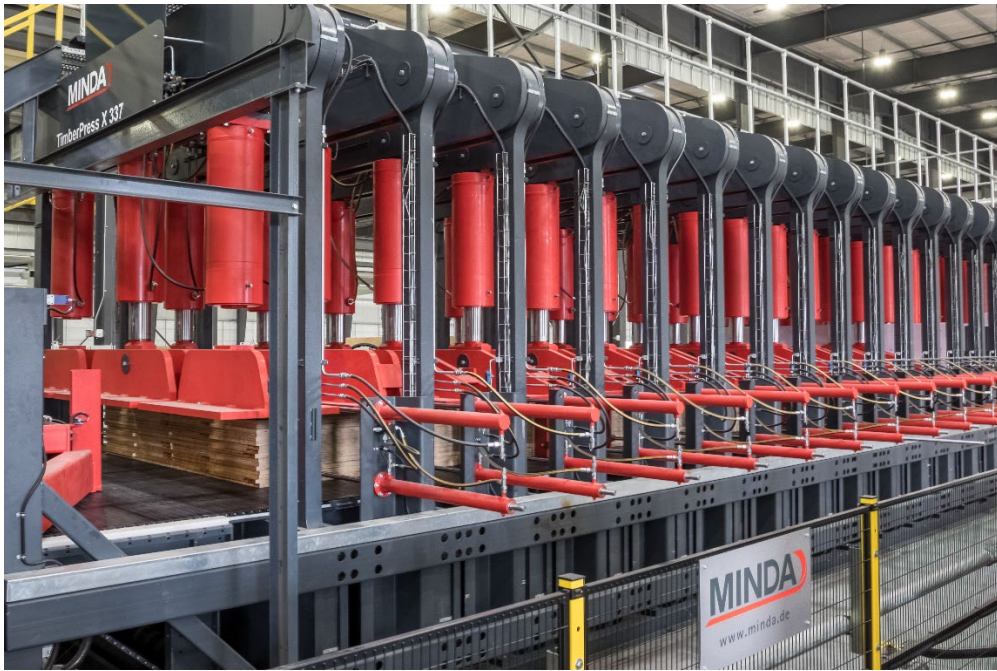
The TimberPress X 337 presses Mass Ply Panels with a pressing pressure of up to 1 N/mm 2
