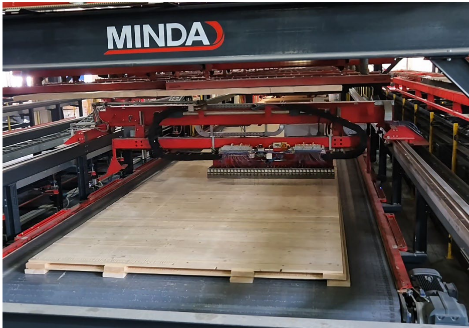
Pulled-out length lamellas to stabilize the cross layer
